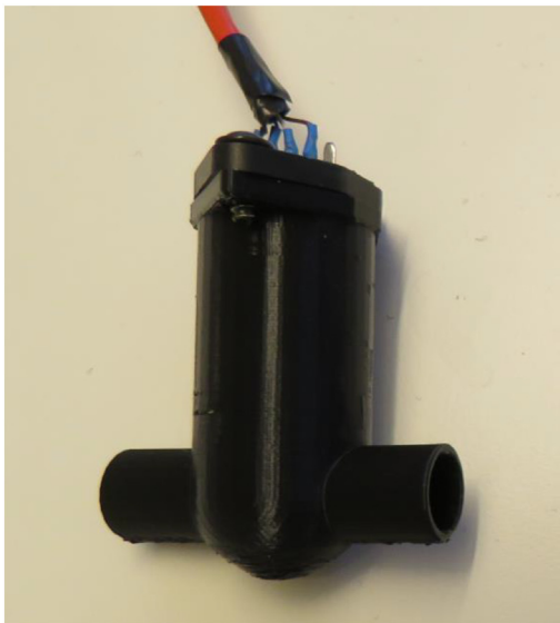
Fig. 3. (Left) 3D printed MAF sensor holder with the MAF sensor core attached (Right) Calibration curve in accordance with the 3D printed MAF sensor holder.
