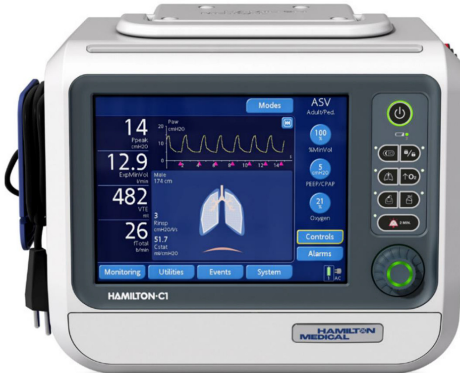
Fig. 5. (Above) GUI of ATMO-Vent with the respiratory parameters on either side in the green background and the settings panel in grey at the bottom. The pressure, flow rate and volume measurements are displayed as real-time plots. (Below) Hamilton-C1 monitor showing essential respiration parameters. (Credits: www.hamilton-medical.com ) This GUI model has been used as a reference for the ATMO-Vent GUI design. (For interpretation of the references to colour in this figure legend, the reader is referred to the web version of this article.)
