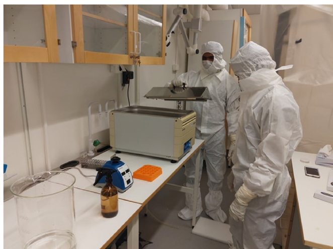
Fig. 6. A very strict garmenting is followed inside the cleanroom tent using ISO 5-certified one-time use bunny suits with double gloves tapped over the sleeves to avoid gapping and contamination release.
