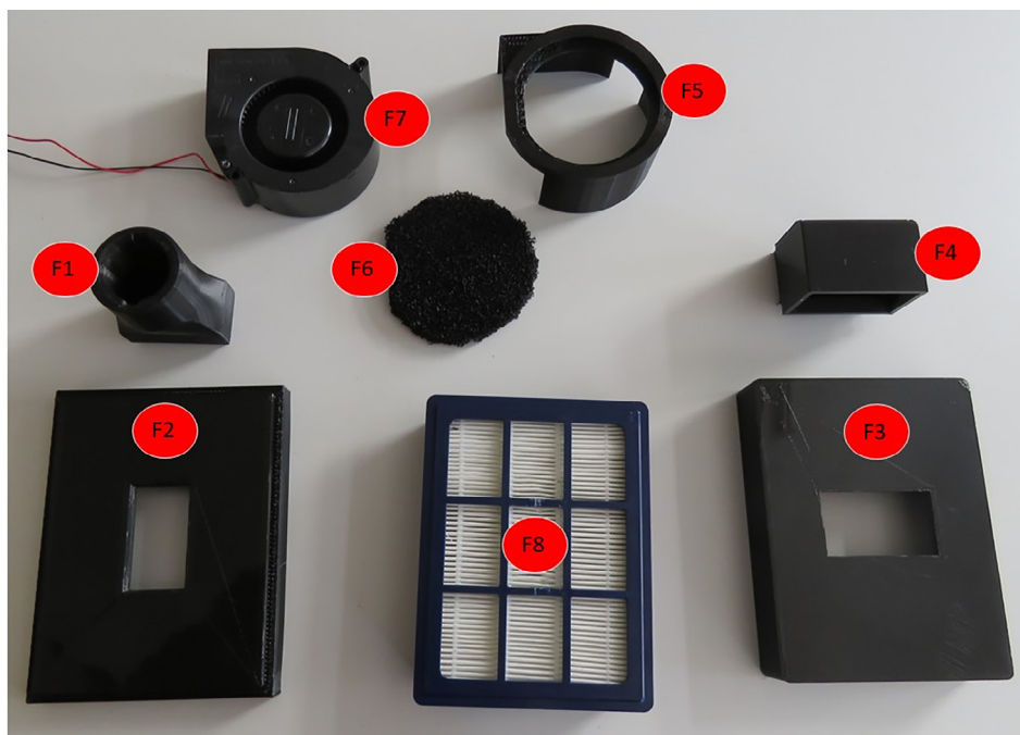
Fig. 8. Components for building the Fan Filter Unit (FFU) are denoted by their designator codes. F1 – Breathing tube adaptor, F2 – HEPA filter outlet adaptor, F3 – HEPA filter inlet adaptor, F4 – right angle duct, F5 – Prefilter holder, F6 – Prefilter, F7 – Centrifugal fan, and F8 – HEPA H14 filter.
