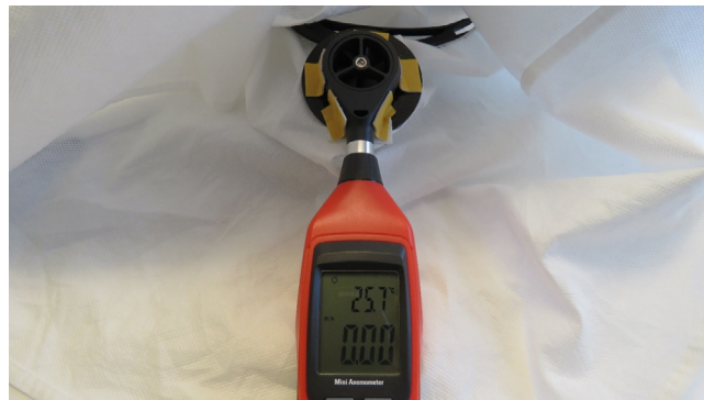
Fig. 18. Experiment setup to determine the air flow inside the hood of PROPER during operation.
