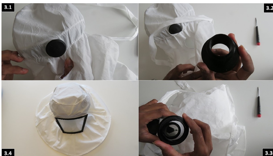
Fig. 7. (Clockwise) Procedure to secure the ratchet knob and hood adaptor. (bottom left) Completed PROPER hood assembly.
