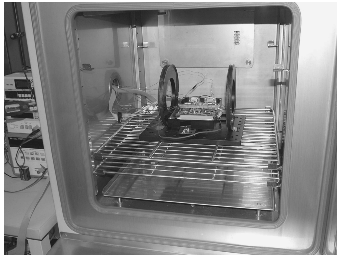
Fig. 13. Temperature characterization of MS with magnetic field created by pair of Helmholtz coils in environmental chamber.
