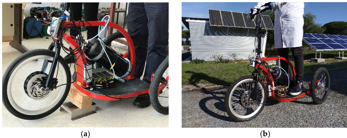
Figure 6. Unipersonal electric vehicle test benches: (a) laboratory dynamic test; (b) road test.
