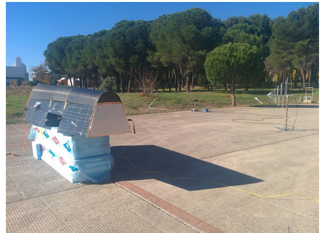
Fig. 6. LLSF OATS test setup. The figure shows a vertically polarized illumination from the starboard of the target.
