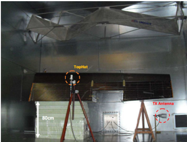
Fig. 5. LLSF RC test setup. The top-hat antenna used for measuring the reference appears in the foreground.
