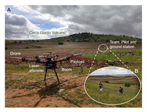
**Figure 4.** (**A**) Hexacopter-type drone provided with a laser altimeter in the landing configuration with the boom horizontal. (**B**) Mobile ground station for tracks longer than 500 m.
