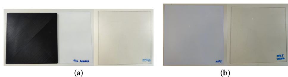
Figure 4. PLA, PETG, HIPS and methacrylate samples: (a) PLA white and black (left) and PETG (right); (b) HIPS (left) and methacrylate (right).
