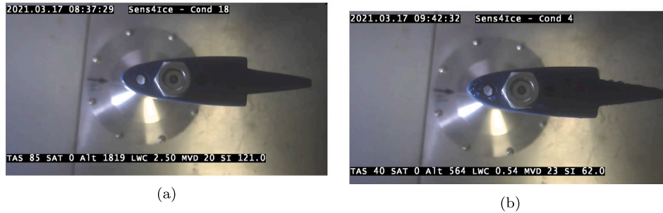
Fig. 9. Test cases without Ice accretion.(a) Test case 18.(b) Test case 4.
