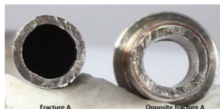
Fig. 2 (b) The fracture surface (A) and its opposite fracture surface
