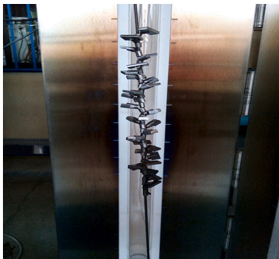
Fig. 2. Image of the test specimens inside the reactor.
