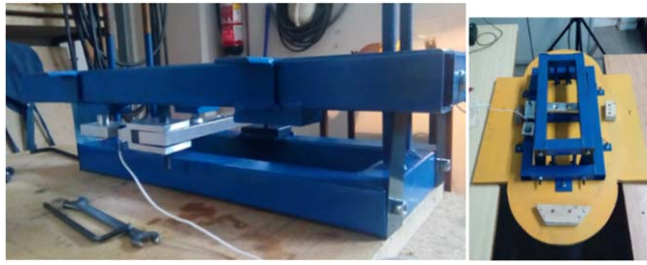
Figure 10. Frames, straps and transmission power mechanism assembled (left). Balance core and wood flooring joined (right).
