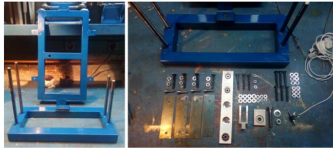
Figure 9. Upper and lower frames (left). Components ready for the assembly (right).
