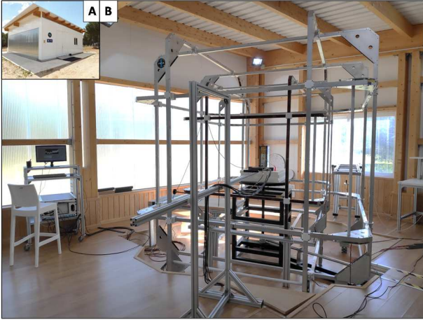
Figure 2. A) INTA Facility; B) three axis Helmholtz coils used during the tests.
