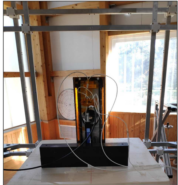
Figure 4. ANSER on-board magnetometer characterization measurement setup.
