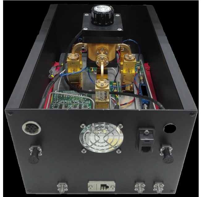
Fig. 6. W -band downconverter for the GACELA receiver. The remotely controlled waveguide switch allowing the selection of one of three W sub-bands is clearly seen at the middle of the box.
