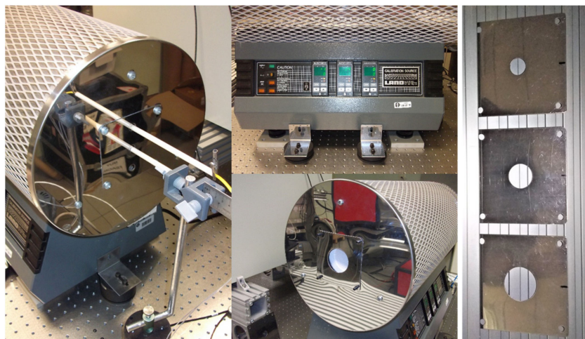
Figure 8. BB source and apertures plates used to validate the SSE characterization procedure.
