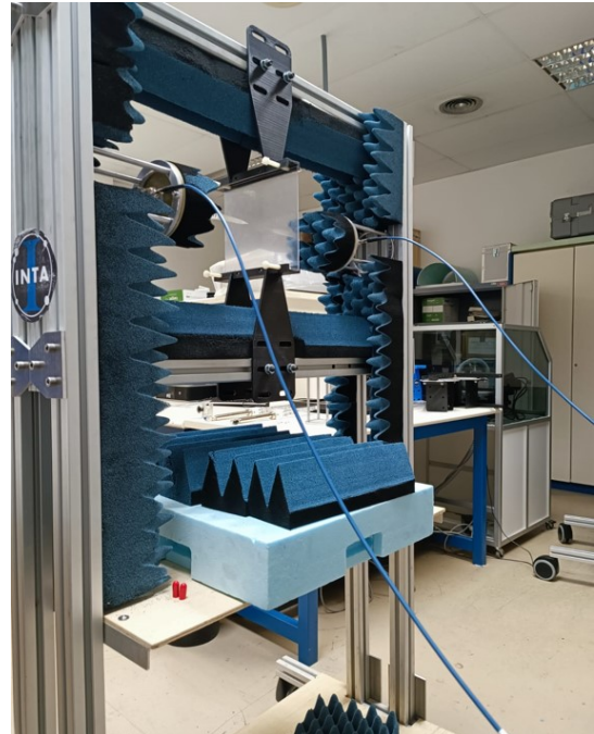
Fig. 1. Free space measurement bench with high precision polyrod antennas.
