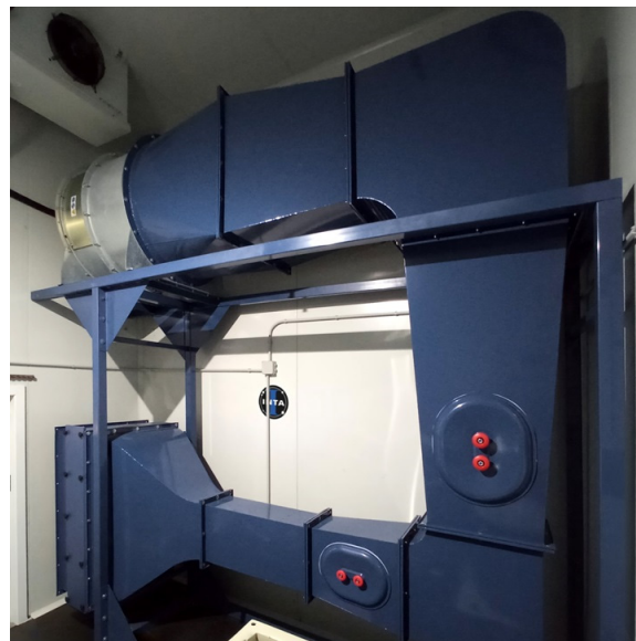
Figure 22. Final IWT in the cold climate chamber.
