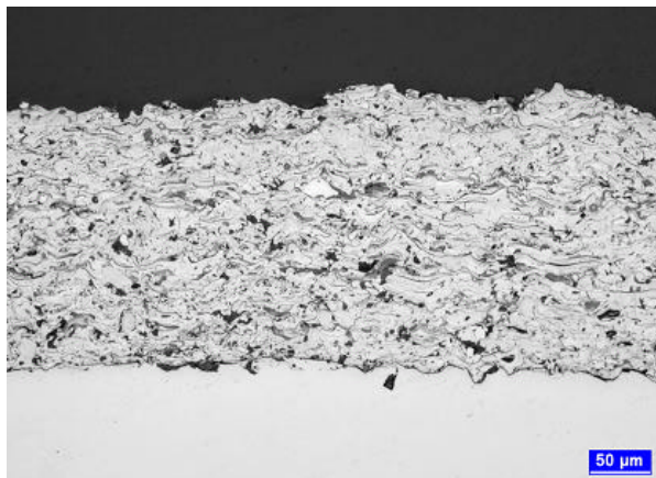
Figure 6. HVOF Ni20Cr coating on P92 substrate.
